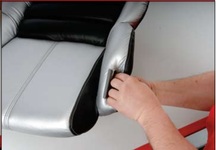
17 ::: Inserting plastic slips attached to cover inside of metal bracket for seat control.
