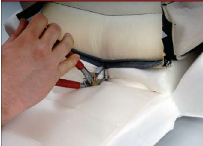
22 ::: Hog ringing seat cover and bladder to wire in foam.
