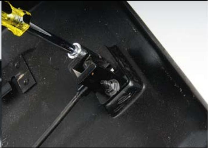
**07** ::: Removing speed nuts from seat back release.
