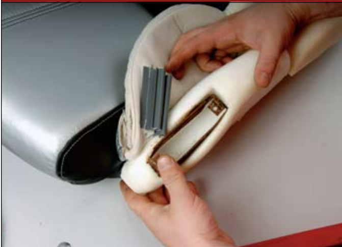
16 ::: Installing metal bracket for seat controls in seat bottom bolster.
