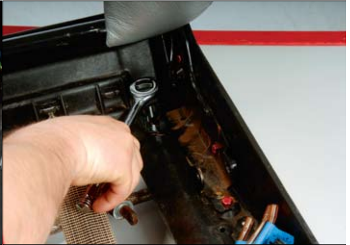
31 ::: Re-installing freshly covered bolsters and brackets.
