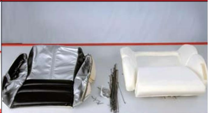
**09** ::: Here are all the supplies needed for completion of the seat bottom.
