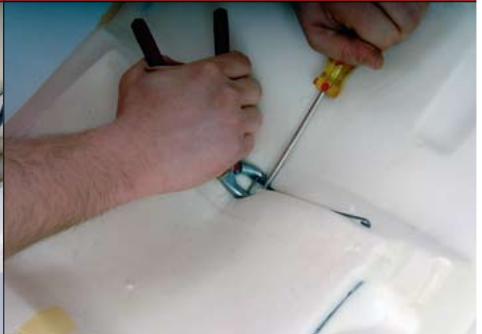
11 ::: Attaching center listing on front side to backing wire on rear of foam with hog rings.
