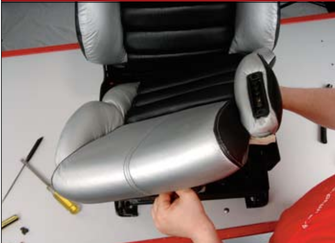
39 ::: Positioning clip to reinstall new seat foam bottom.
