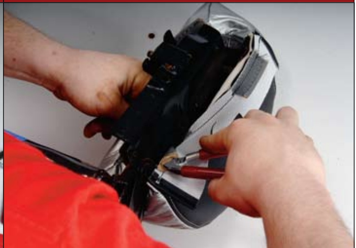
27 ::: Hog ring outer bolster cover over metal frame.
