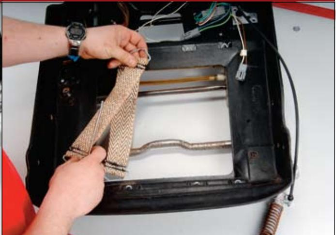
**29** ::: Removing seat bottom trapeze from mounting brackets.
