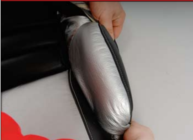
14 ::: Wrapping seat bolsters in preparation for final hog ringing.
