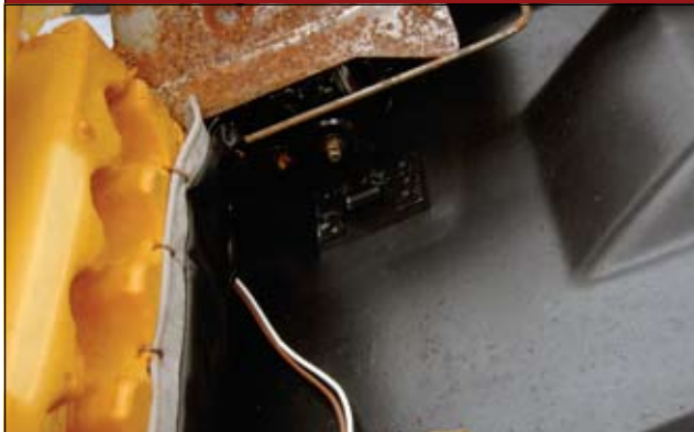
02 ::: Next he unclips the wire of the seat frame.
