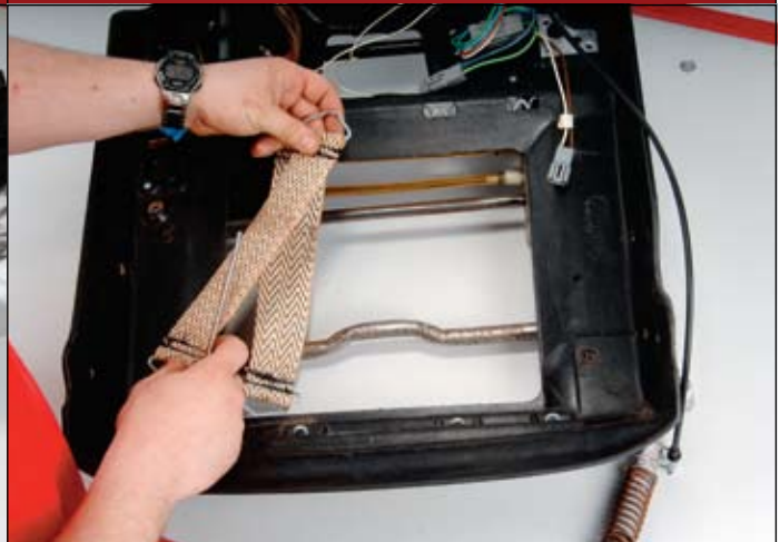
29 ::: Removing seat bottom trapeze from mounting brackets.
