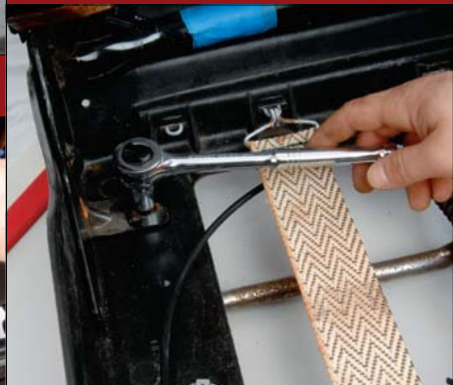
05 ::: Next, he removes the bolts located in brackets for seat bolsters.
