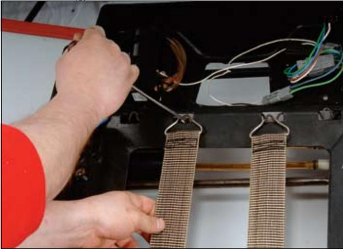
**30** ::: Installing new seat bottom trapeze kit.
