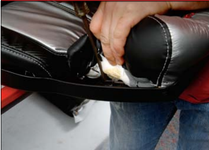
34 ::: Attaching headrest wire to clip in seat frame.
