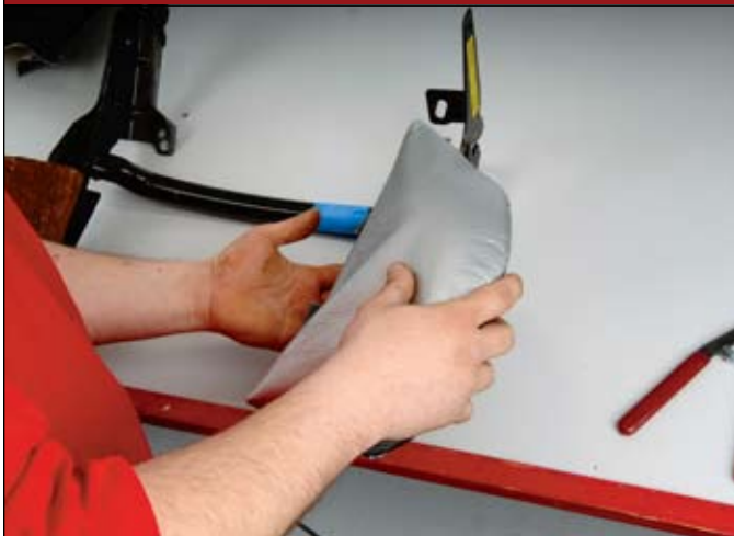
26 ::: Installing bolster cover over metal frame.
