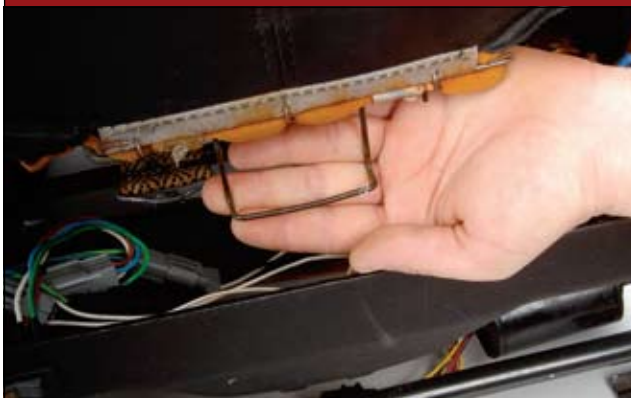
03 ::: Unattaching clip located on the front of seat bottom.
