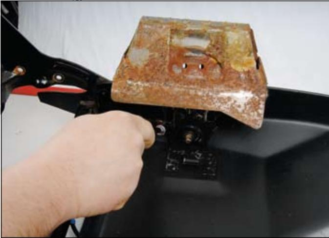
**06** ::: Removing bolts from seat bolsters located in seat back.
