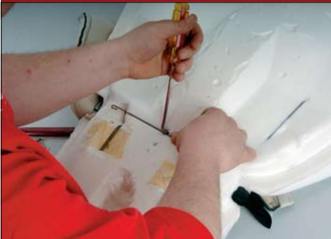
**20** ::: Pulling extension clips through to backing. Wire on back side of foam.
