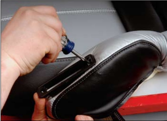
36 ::: Installing bezel surround over seat control.
