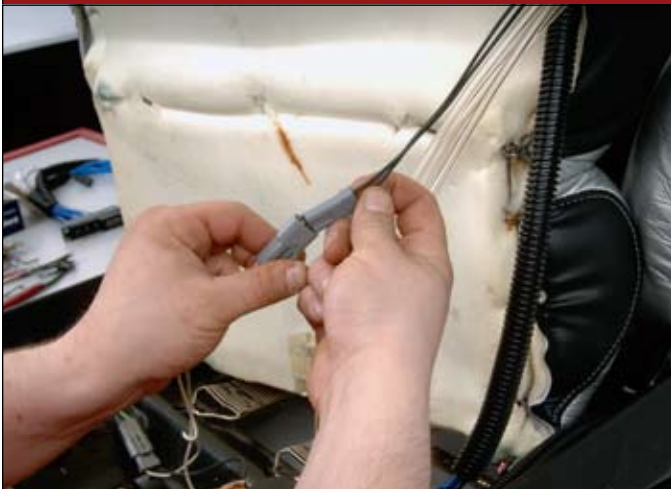
38 ::: Hooking up seat control wiring harness.
