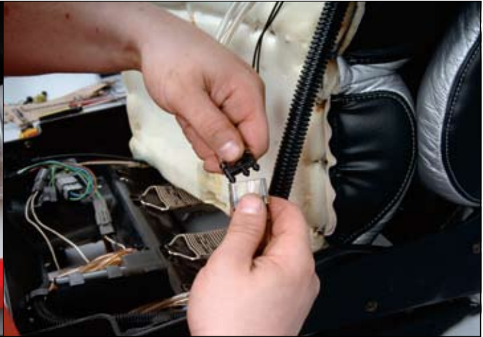
37 ::: Hooking up seat bladder control hoses.
