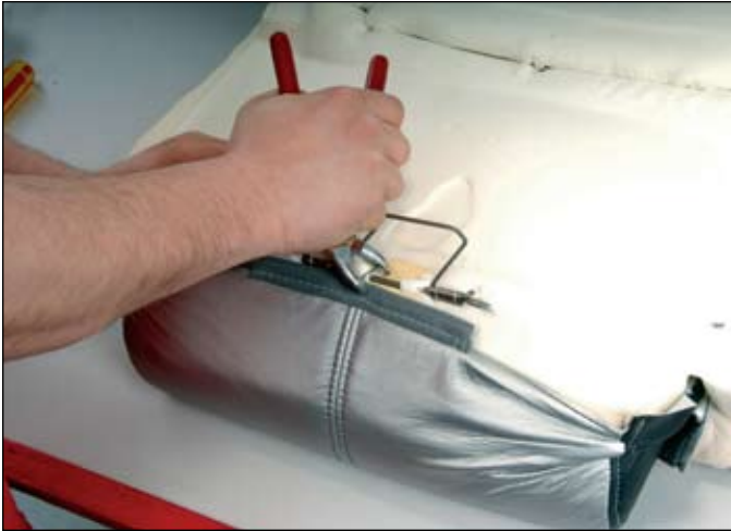
12 ::: Attaching front of cover to wires in formed foam with hog rings.
