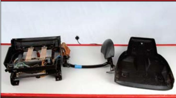
**08** ::: Seat bolsters are now removed for easier installation.
