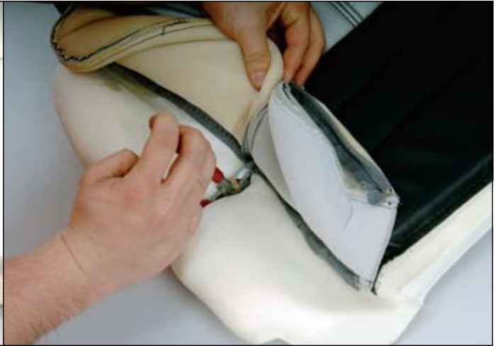
13 ::: Hog ringing inside of seat bolsters to wipe in foam.
