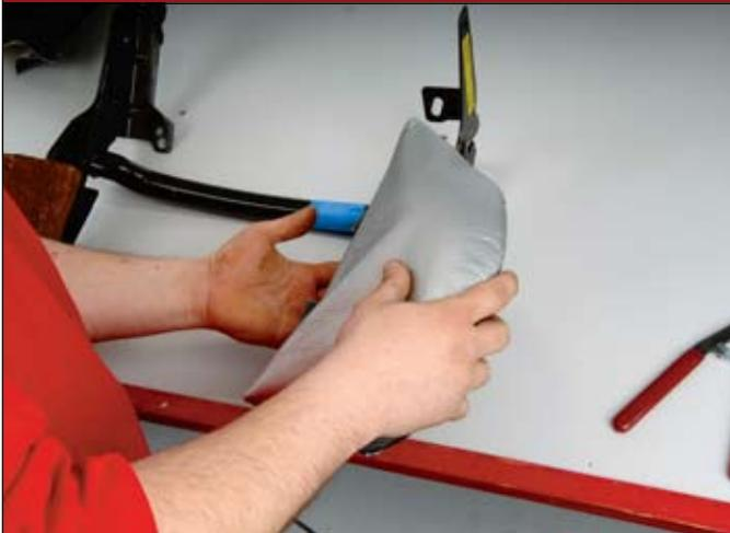
**26** ::: Installing bolster cover over metal frame.
