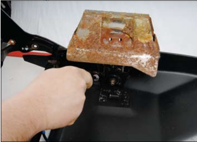
06 ::: Removing bolts from seat bolsters located in seat back.
