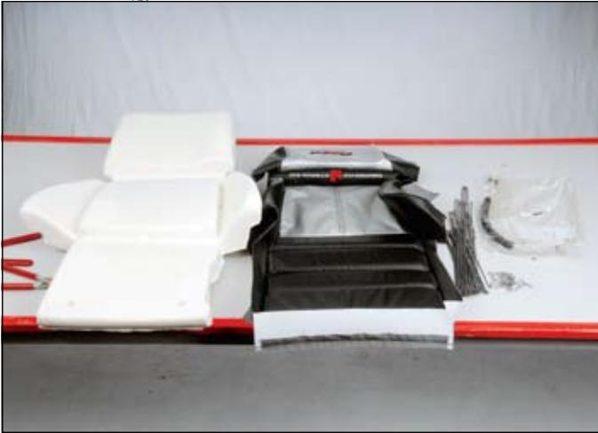
**18** ::: Here is all hardware needed for installing the seat back cover to the seat foam.
