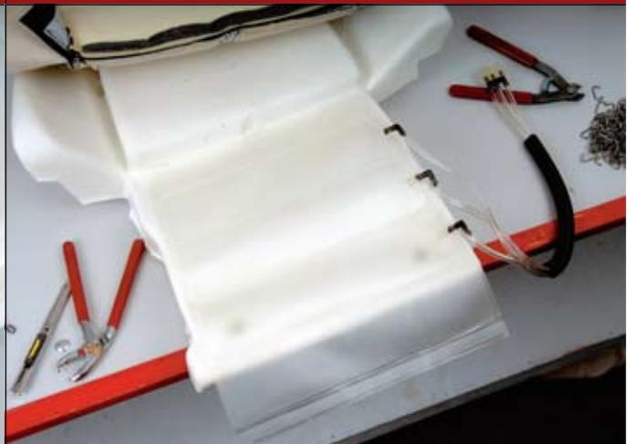
**21** ::: Installing seat bladders to lower seat foam.
