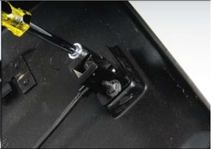
07 ::: Removing speed nuts from seat back release.
