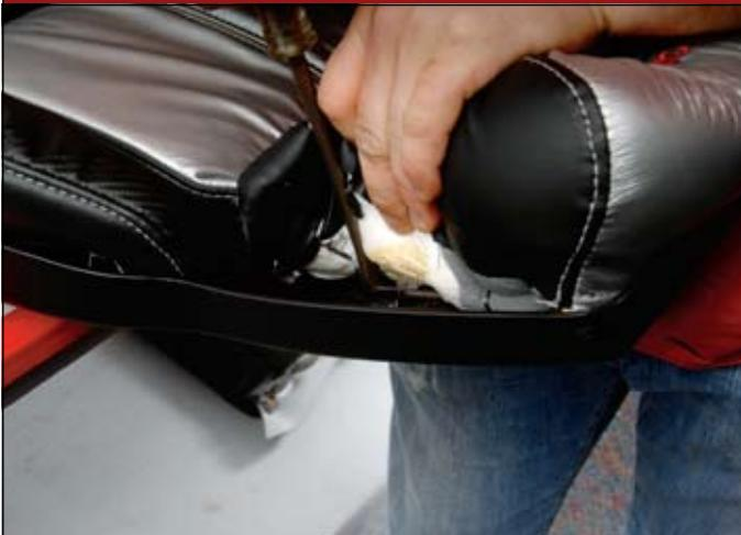
**34** ::: Attaching headrest wire to clip in seat frame.
