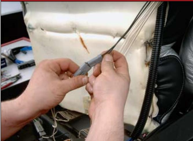
**38** ::: Hooking up seat control wiring harness.
