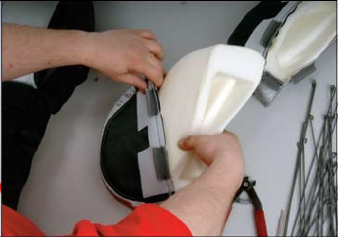
**25** ::: Inserting foam into bolster covers.
