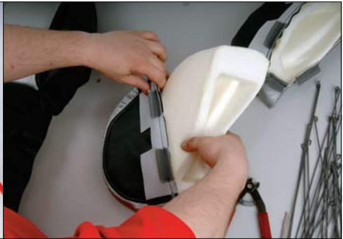
25 ::: Inserting foam into bolster covers.
