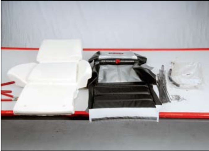
18 ::: Here is all hardware needed for installing the seat back cover to the seat foam.
