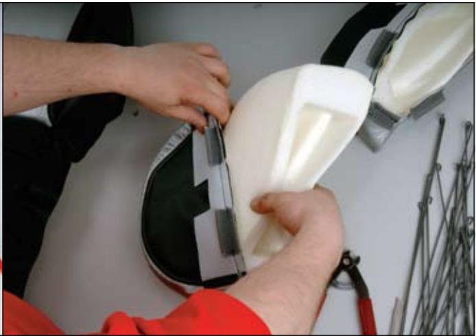
**25** ::: Inserting foam into bolster covers.
