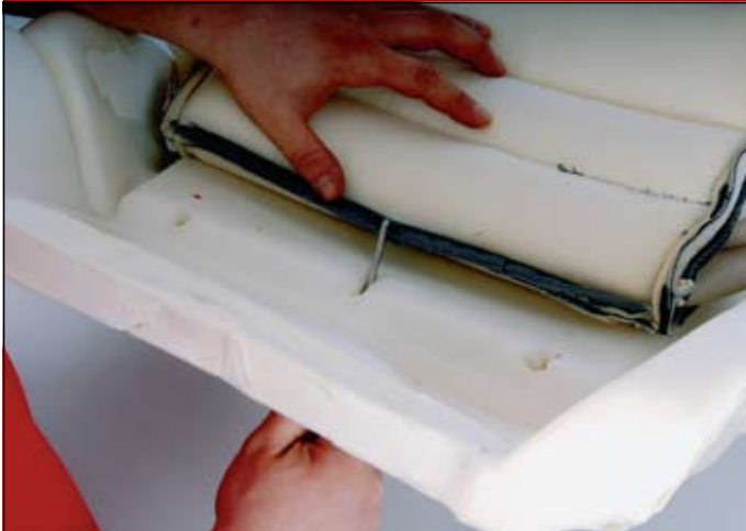
10 ::: Positioning and preparing to hog ring center listing on the seat bottom.
