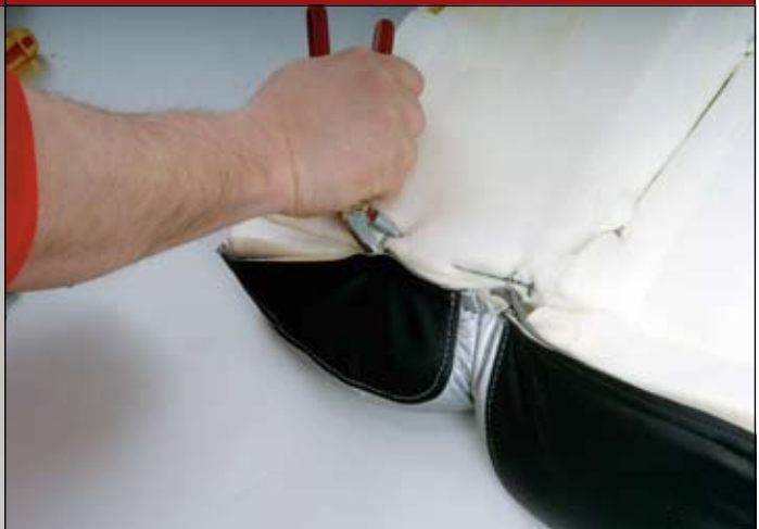
15 ::: Final hog ringing process for bolsters on bottom side of foam.
