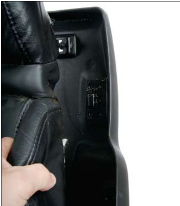
01 ::: First, Matt unclips the seat back cushion from the seat frame.
