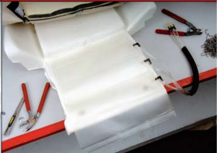
21 ::: Installing seat bladders to lower seat foam.
