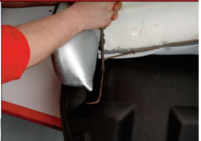
33 ::: Attaching headrest wire to clip in seat frame.
